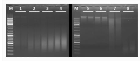
Figure 11: Gel electrophoretic separation of DNA purifed from fluid or solid food samples as indicated in the table above
