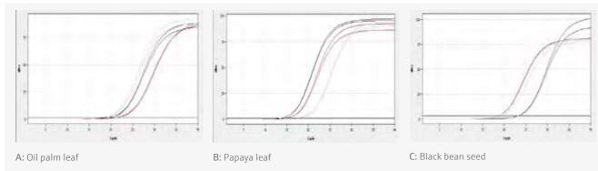
Figure 6: Depending on the starting material, the three lysis buffer system of the innuPREP Plant DNA Kit simplifies and speeds up the extraction process. The real-time plots show the influence of lysis on the final amplification results. Black: Lysis buffer CBV. Red: Lysis buffer OPT. Gray: Lysis buffer SLS.
